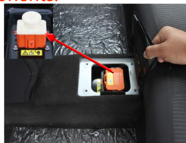
Service switch and protective plug
