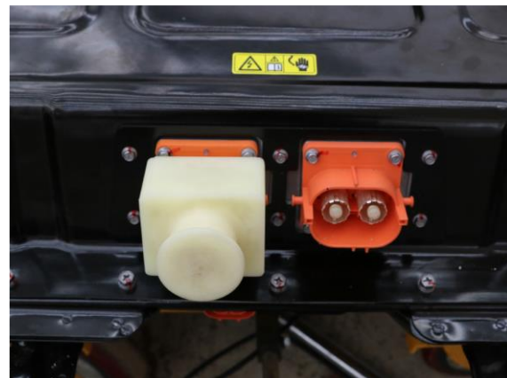
Traction battery wire harness socket plug
