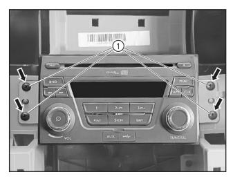
Tighten the fixing screw (1) of CD player with the Phillips screwdriver.
