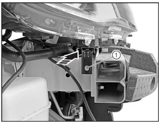
Align the bolt holes (1), install the headlamp assembly bracket on the body, and then install the fixing bolts (M6X20) of headlamp assembly bracket.
