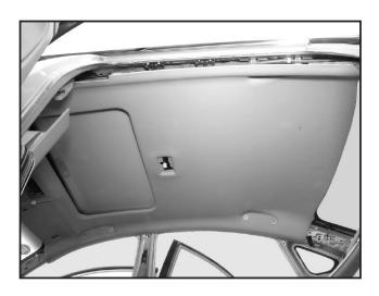
Gently pull the roof inner trim panel downwards so as to detach it from the rear clips, and take the roof inner trim panel slowly out from the rear door.
