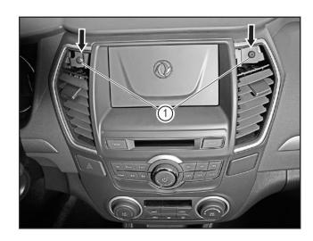
Tighten the fixing screws (1) of the central panel frame with the Phillips screwdriver.
