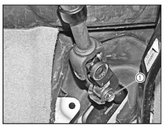
Tighten the connecting bolt (1) between lower steering column and steering gear with the 12mm socket to 35.8N·m. Check for missed installation of lock washer.
