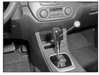
Inset the shift lever (1) into the mounting end with the large end facing forward, and then clip it firmly.
