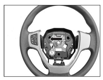
Install the garnish onto the steering wheel and insert the horn connector (1) in the direction as indicate by the arrow.
