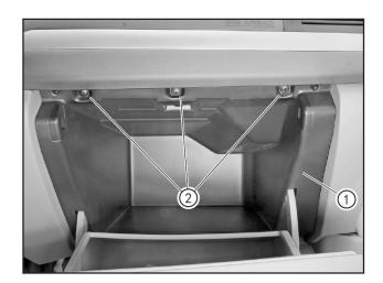
• Refit the glove box assembly (1), and tighten the 3 fixing screws (2) of the glove box assembly .
