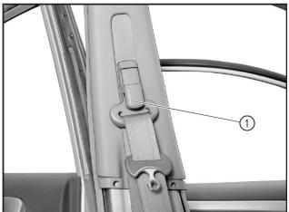
Pry up the shoulder belt fixing guide ring cover (1) with the interior trim removal tool (BF1102).
