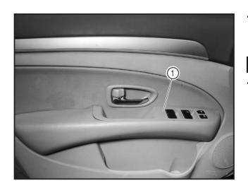
Install the front end of the door electric main switch panel (1) into the door protective plate first, and then press the door electric main switch panel into position.
