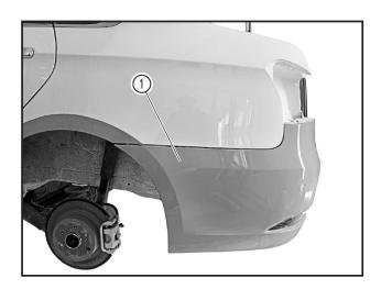
Hold up the wheel arch part of rear bumper (1) and pull it outward gently so as to separate it from the pawl of rear bumper side bracket.
