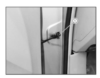
Tear off the sealing film of the door wire harness on the door post, pull the door wire harness connector out of the door post, and press the connector clip A, and disconnect the door connector (1).
