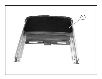
• Two operators are required to cooperate to lift off the sunroof assembly (1).
