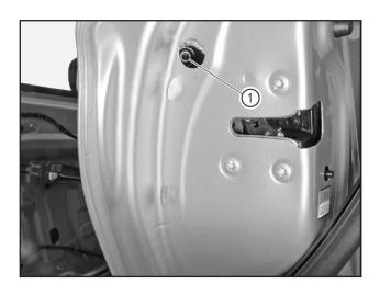
Remove the fixing screw (1) of the outside handle trim cover with the T30 screwdriver bit.
