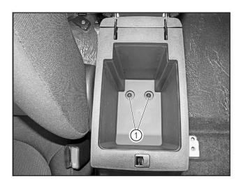
• Tighten the 2 fixing screws (1) in the center armrest box with the Phillips screwdriver.
