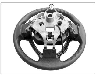
• Refit the 2 fixing screws (1) of the garnish.
