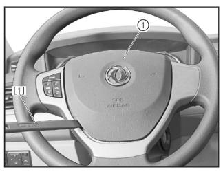
Pry up the driver frontal airbag (1) with the interior trim removal tool (BF1102) [1].
