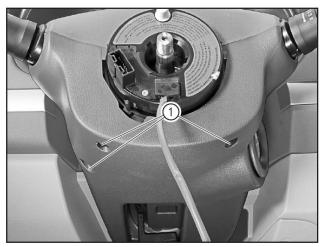
Remove the fixing screws (1) from the upper and lower shrouds of steering column with the Phillips screwdriver.
