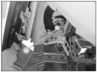
Connect the airbag connector (1) and confirm that it is locked effectively.
