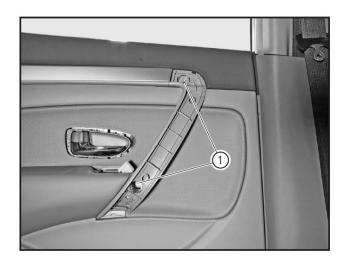
Remove the fixing bolts (1) of rear door inner protective plate with the 10mm socket.
