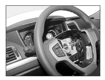
Use the 19mm socket to tighten the steering wheel lock nuts (1) to 33N·m.
