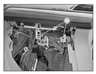
Tighten the 2 lower fixing bolts (1) (M8×20) of the front passenger's airbag with the 12mm socket to 24.5N⋅m.
