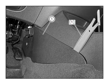
Remove the console left protective plate (1) with the interior trim removal tool (BF1102) [1].
