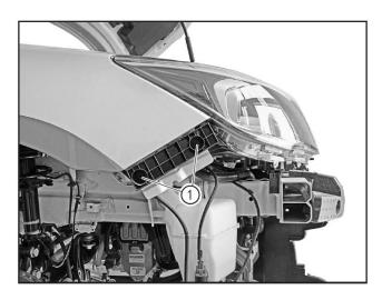
Remove the fixing screw (1) of the front bumper bracket with the 10mm socket.
