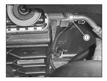
Remove the fixing nut (1) of A/C compressor high-pressure pipe (condenser side) with the 10mm open-end wrench.
