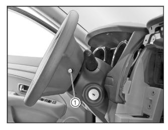
Tighten the 2 airbag fixing bolts (1) under the steering wheel (1 for each side) with the T30 screwdriver bit to 10N·m.
