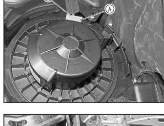
Press the connector clip A, and disconnect the fan connector (1) outwards.
