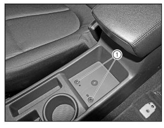
Tighten the 2 fixing screws (1) at the upper part of the console with the Phillips screwdriver.
