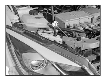
Align the bolt holes (1) on the upper part of headlamp, and install the 2 upper fixing bolts (M6X20) of the headlamp.
