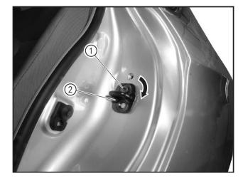
Loosen the fixing screw (1) of the rear door lock catch with the T30 screwdriver bit, and then rotate the rear door lock catch (2) downwards.
