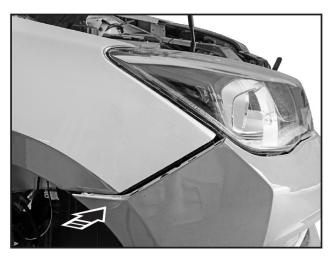
Two workers are required for cooperation: align the front bumper bracket pawl with the hole, and install the front bumper properly.
