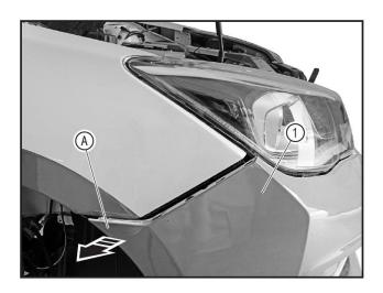
Lift the side of front bumper and pull it outward gently at position (A) so as to separate the side from the bracket pawl, and take the bumper (1) off the body.
