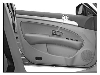
Clamp the inside handle trim cover (1) to the mounting surface on the door protective plate with the positioning clips aligned.
