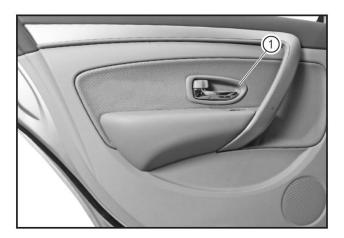
Press fit the inside handle trim cover (1) into the mounting holes on the door inner protective plate in place after alignment.
