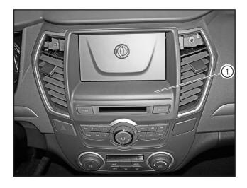
Press fit the central panel frame (1) in place after aligning the clips thereon with the fixing points on the instrument panel.
