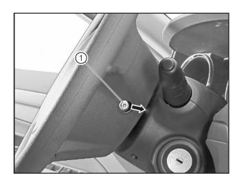
Remove the fixing screw (1) of the driver frontal airbag with the T30 screwdriver bit.
