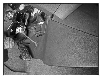
• Remove the fixing clip (1) of console left protective plate with the Phillips screwdriver.
