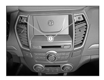
Remove the fixing screws (1) of the central panel frame with the Phillips screwdriver.
