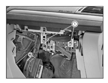
Remove the 2 lower fixing bolts (1) (M8X20) of the front passenger's airbag with the 12mm socket, and take the airbag down.
