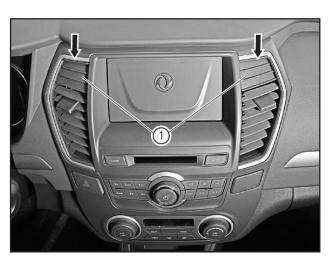
Press fit the fixing screw cap (1) of the center panel frame in place.
