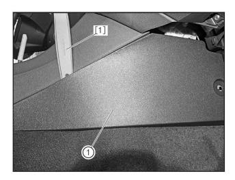
Remove the console right protective plate (1) with the interior trim removal tool (BF1102) [1].
