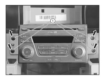
Remove the fixing screw (1) of CD player with the Phillips screwdriver.
