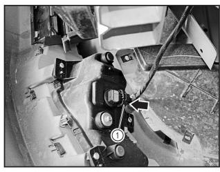
Refit the front fog lamp connector (1) with the jack aligned.
