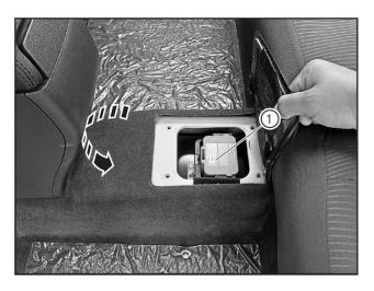
• Refit the service switch (1). (Refer to "Removal and Refitting of Service Switch" in "Traction Battery")
