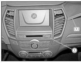
Remove the central panel frame (1) with the interior trim removal tool (BF1102) [1].
