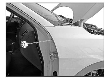
• Align the bolt holes (1) and install the fender fixing bolts (M6X15).
