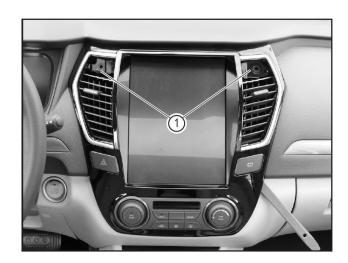
Remove the fixing screws (1) of the central panel frame with the Phillips screwdriver.
