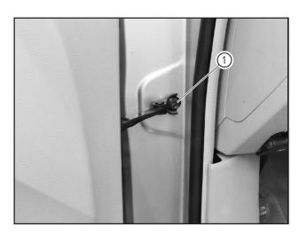
Tighten the fixing bolt (1) of the door stopper with the 10mm socket.
