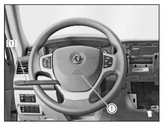
Pry open the driver's airbag (1) with the interior trim removal tool [1].
