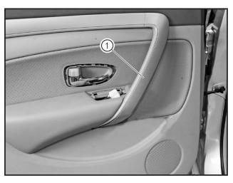
Install the rear door handle cover (1) into the mounting hole after alignment.
