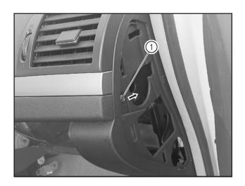
Remove the instrument panel fixing screw (1) with the Phillips screwdriver. (1 pcs on each side)
