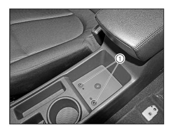
Remove the 2 fixing screws (1) at the upper part of the console with the Phillips screwdriver.
