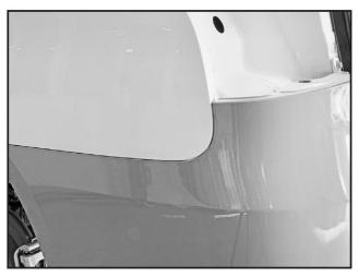
Check whether the gap of the rear bumper with the rear fender and the trunk lid meets the requirements.
