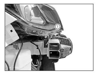
Remove the fixing bolt (1) (M6X20) of headlamp assembly bracket with the 10mm socket.
