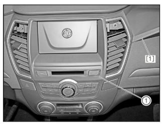
Remove the central panel frame (1) by the interior trim removal tool (BF1102) [1].
