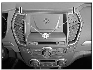
Press fit the fixing screw cap (1) of the center panel frame in place.
