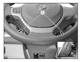
Remove the airbag fixing screw cap (1) under the steering wheel with the interior trim removal tool (BF1102).
