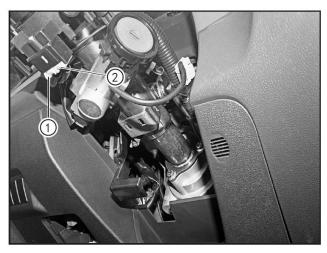
Disconnect the airbag connector (1) and horn connector (2) below the rotary switch and combination switch assembly.
