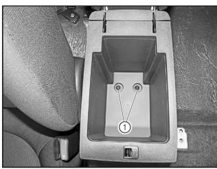
• Remove the 2 fixing screws (1) in the center armrest box with the Phillips screwdriver.
