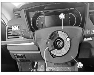
Pry open the upper shroud (1) and lower shroud (2) from the steering column by using the interior trim removal tool (BF1102) [1].
