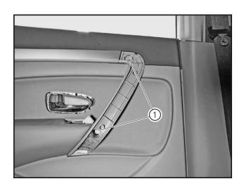
Tighten the fixing bolts (1) of rear door inner protective plate with the 10mm socket.
