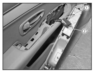
• Connect the central locking connector (1) and the power window switch connector (2) into position.
