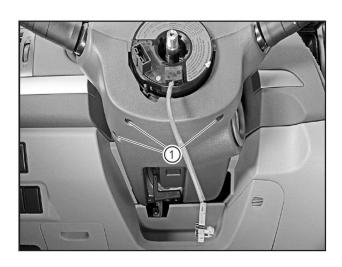
Remove 3 fixing bolts (1) for lower shroud of steering column with the Phillips screwdriver.
